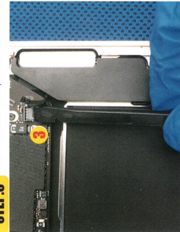
STEP:8 Disconnect the loudspeaker interface
