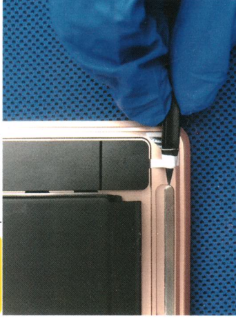
STEP:11 Slowly pull out the loudspeaker adhesive tape at both ends
