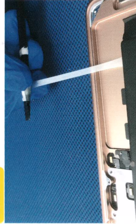
STEP:14 Pry up the battery adhesive tape
