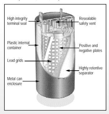
Gasses produced in normal overcharge are recombined within the cell. A re-sealable bunsen valve is incorporated to permit gas venting in the case of abusive overcharge.
