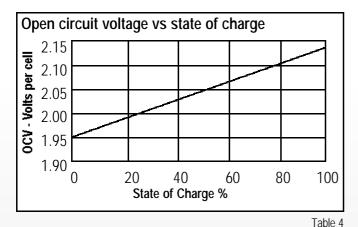
Note:- This curve is accurate to within 20% of the cell's rated capacity, if it has not been charged or discharged within the past 24 hours. The curve is accurate to within 5% if the cell has not seen any activity, charge or discharge, for the past 5 days.
